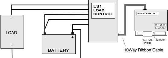
PLA and LS1 Connection (Separate power connection to PLA is not required )
